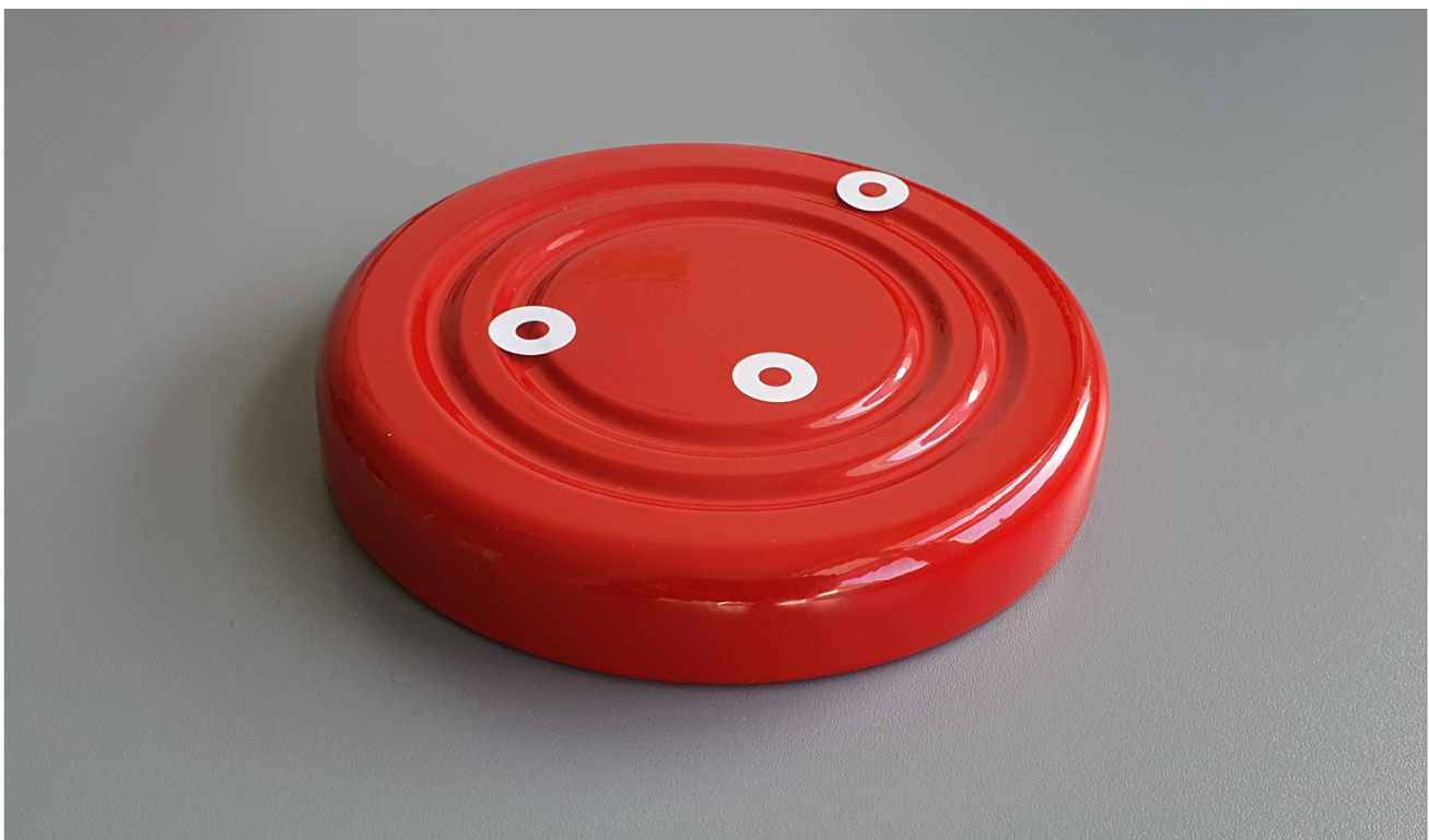
Figure 19: Ring stickers marking the points where the reference coating thickness was measured
