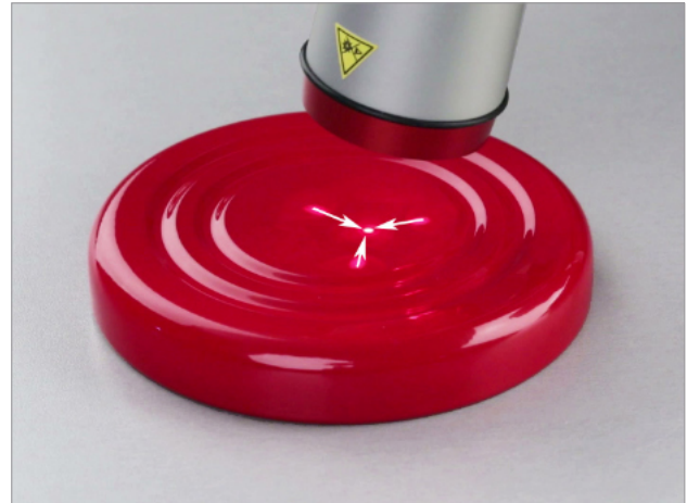
Fig. 17: Align the three light dots to a single point
