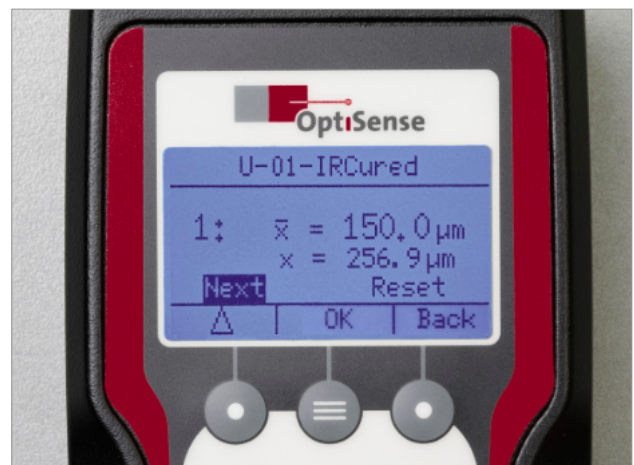
Fig. 25: Enter the actual coating thickness
