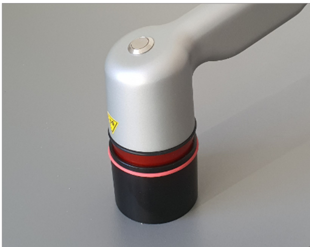
Fig. 13: Automatic self-test with gray glass reference
