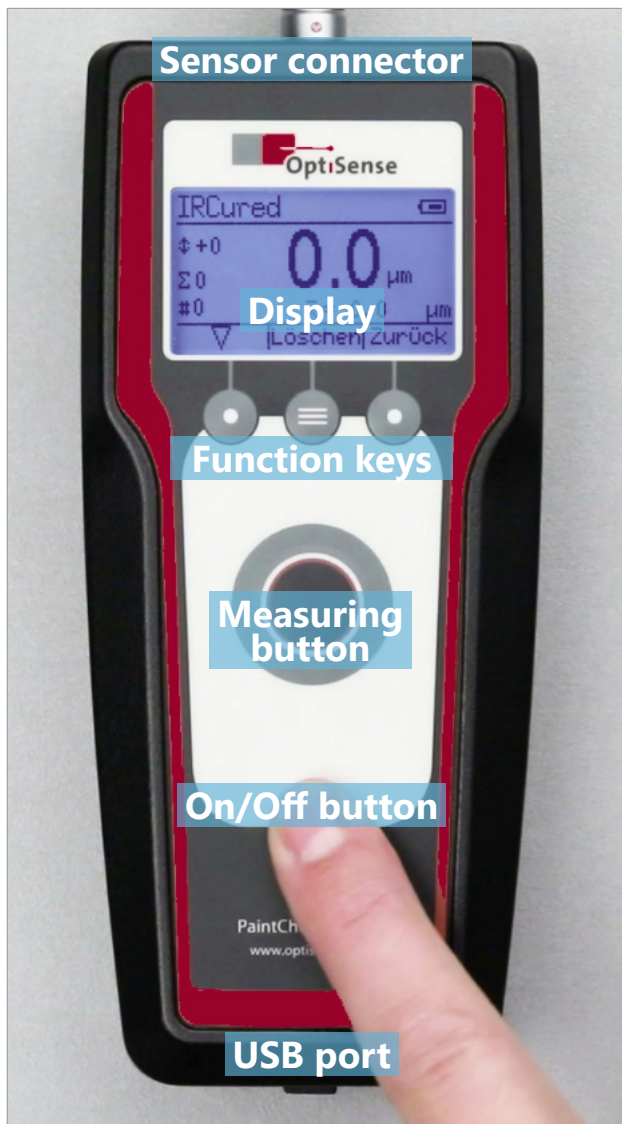
Fig. 9: PaintChecker Mobile operation
