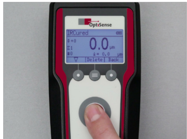
Fig. 8: Switching the device on and off
