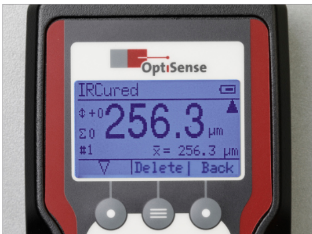
Fig. 23: Measurement exceeds limit
